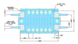
NOTES: 1. TRACE WIDTH IS SHOWN FOR OAK-602, WITH DIELECTRIC THICKNESS .022"±.0015". COPPER: 1/2 Oz. EACH SIDE. FOR OTHER MATERIALS TRACE WIDTH MAY NEED TO BE MODIFIED. 2. BOTTOM SIDE OF THE PCB IS CONTINUOUS GROUND PLANE. DENOTES PCB COPPER LAYOUT WITH SMOBC (CONTENT WICK OWER BASE CORPER) (SOLDER MASK OVER BARE COPPER)
