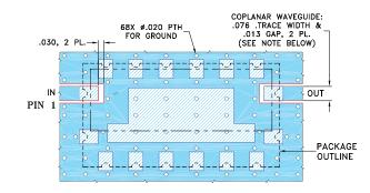
NOTE: 1. COPLANAR WAVEGUIDE PARAMETERS ARE SHOWN FOR ROGERS R04350B WITH DIELECTRIC THICKNESS .060" ± .004"; COPPER: 1/2 OZ. EACH SIDE. FOR OTHER MATERIALS TRACE WIDTH MAY NEED TO BE MODIFIED. 2. BOTTOM SIDE OF THE PCB IS CONTINUOUS GROUND PLANE.
