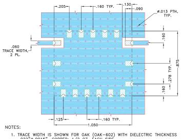
TRACE WIDTH IS SHOWN FOR OAK (OAK-602) WITH DIELECTRIC THICKNESS .022"±.0015". COPPER: 1/2 OZ. EACH SIDE. FOR OTHER MATERIALS TRACE WIDTH MAY NEED TO BE MODIFIED.
