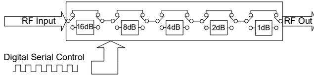
The DAT-3175A-SP+ serial interface consists of 5 control bits that select the desired attenuation state, as shown in Table 1: Truth Table
