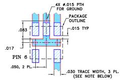
NOTES: 1. TRACE WIDTH IS SHOWN FOR ROGERS RO4350B WITH DIELECTRIC THICKNESS 0.030" ± 0.002"; COPPER: 1/2 OZ. EACH SIDE. FOR OTHER MATERIALS TRACE WIDTH MAY NEED TO BE MODIFIED. 2. BOTTOM SIDE OF THE PCB IS CONTINUOUS GROUND PLANE.
