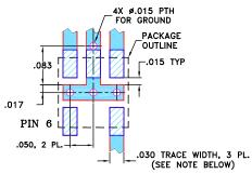
NOTES: 1. TRACE WIDTH IS SHOWN FOR ROGERS RO4350B WITH DIELECTRIC THICKNESS 0.030" ± 0.002"; COPPER: 1/2 OZ. EACH SIDE. FOR OTHER MATERIALS TRACE WIDTH MAY NEED TO BE MODIFIED. 2. BOTTOM SIDE OF THE PCB IS CONTINUOUS GROUND PLANE.
