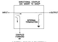
ELECTRICAL SCHEMATIC IS FOR DIRECTIONAL COUPLER WITH INTERNAL TRANSFORMER(S) THA POLITES DC FROM RF PORTS TO GROUND REV. A M151107 ED-8967A/1 DBTC-13-5-75LX+ WZ/CP/AM 190821
