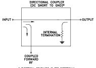
ELECTRICAL SCHEMATIC IS FOR DIRECTIONAL COUPLER WITH INTERNAL TRANSFORMER(S) THAT ROUTES DC FROM RF PORTS TO GROUND. REV. A M151107 ED-10793A/1 DBTC-20-4LX+ WP/CP/AM 190827 Page 1 of 2
