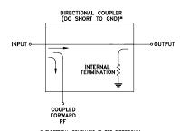
ELECTRICAL SCHEMATIC IS FOR DIRECTIONAL COUPLER WITH INTERNAL TRANSFORMER(S) THA POLITES DC FROM RF PORTS TO GROUND
