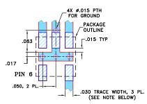
NOTES: 1. TRACE WIDTH IS SHOWN FOR ROGERS RO4350B WITH DIELECTRIC THICKNESS 0.030" ± 0.002"; COPPER: 1/2 0Z. EACH SIDE. FOR OTHER MATERIALS TRACE WIDTH MAY NEED TO BE MODIFIED. 2. BOTTOM SIDE OF THE PCB IS CONTINUOUS GRO
