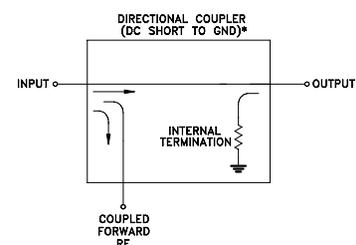
\* ELECTRICAL SCHEMATIC IS FOR DIRECTIONAL COUPLER WITH INTERNAL TRANSFORMER(S) THAT ROUTES DC FROM RF PORTS TO GROUND.
