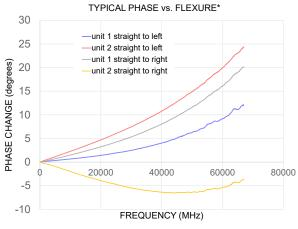
Typical phase change over flexure performed on E67-1M-EMEM+ by wrapping cable 360° around 4" radii mandrels referenced to normalized straight position.
