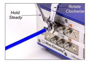
NOTE: Mini-Circuits recommends using a 5/16-inch open end wrench calibrated to 8 inch-pounds maximum torque to prevent damage due to over-torqueing the connector.
