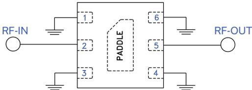
Fig 1. Block Diagram of Test Circuit used for characterization. Test Board TB-EQY-5-283+
