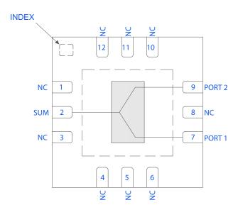
Figure 1. GP2S1A+ Functional Diagram
