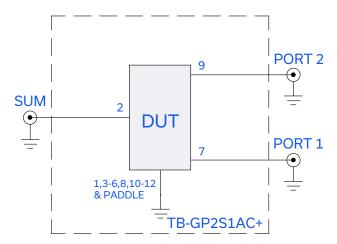
Figure 2. GP2S1A+ Characterization and Application Circuit.
