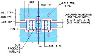
NOTES: 1. COPLANAR WAVEGUIDE PARAMETERS ARE SHOWN FOR ROGERS R04350B WITH THICKNESS .020" ± .0015". COPPER: 1/2 OZ. EACH SIDE. FOR OTHER MATERIALS TRACE WIDTH & GAP MAY NEED TO BE MODIFIED.
