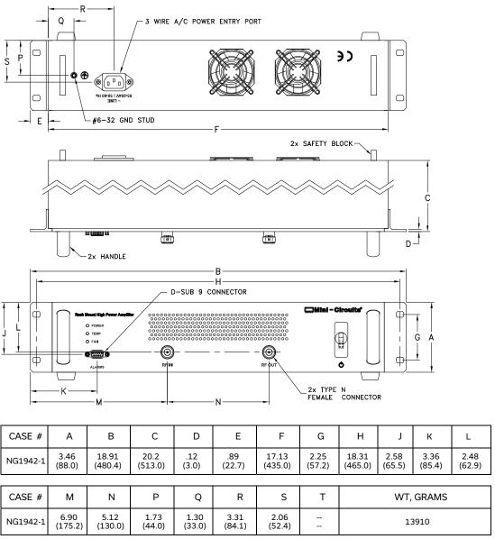
Dimensions are in inches (mm). Tolerances: 2PI. ±.03; 3PI. ±.015 inch
