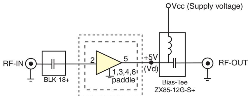
**Fig 1.** Block Diagram of Test Circuit used for characterization. (DUT soldered on Mini-Circuits Characterization test board TB-640+) Gain, Return loss, Output power at 1dB compression (P1 dB) , output IP3 (OIP3) and noise figure measured using Agilent’s N5242A PNA-X microwave network analyzer.
