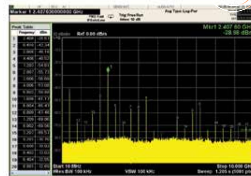
IF output reflection spectrum without filter
