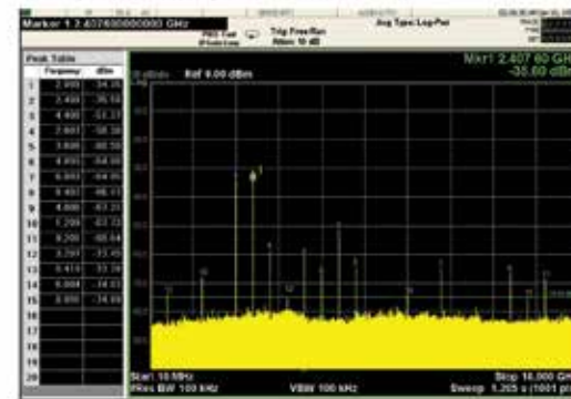
IF output reflection spectrum with conventional filter
