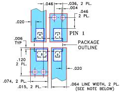
NOTES: 1. TRACE WIDTH IS SHOWN FOR ROGERS RO4350B WITH DIELECTRIC THICKNESS .030"  $\pm$  .002"; COPPER: 1/2 OZ. EACH SIDE. FOR OTHER MATERIALS TRACE WIDTH MAY NEED TO BE MODIFIED. 2. BOTTOM SIDE OF THE PCB IS CONTINUOUS GROUND PLANE.
