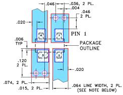
$\underline{\text{NOTES:}}$  1. TRACE WIDTH IS SHOWN FOR ROGERS RO4350B WITH DIELECTRIC THICKNESS .030"  $\pm$  .002"; COPPER: 1/2 OZ. EACH SIDE. FOR OTHER MATERIALS TRACE WIDTH MAY NEED TO BE MODIFIED.
