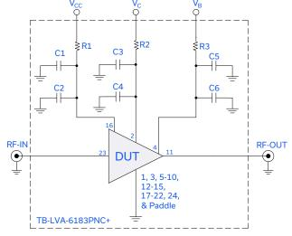
Figure 2. LVA-6183PN+ Characterization and Application Circuit
