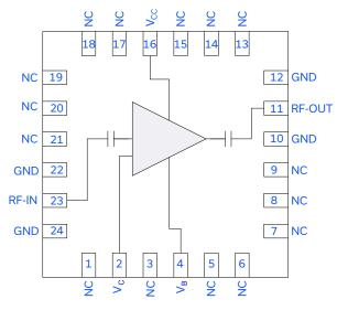
Figure 1. LVA-6183PN+ Functional Diagram
