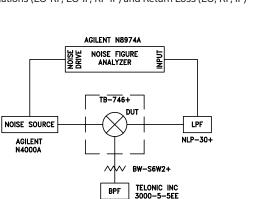
Block Diagram of Test Circuit used for characterization of Noise Figure.
