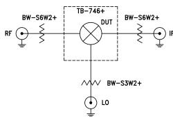
Figure 1A. Block Diagram of Test Circuit used for characterization of Conversion Loss, Isolations (LO-RF, LO-IF, RF-IF) and Return Loss (LO, RF, IF)
