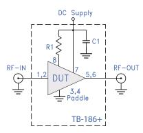
Fig 1. Block Diagram of Test Circuit used for characterization. (DUT soldered on Mini-Circuits Characterization test board TB-186+)
