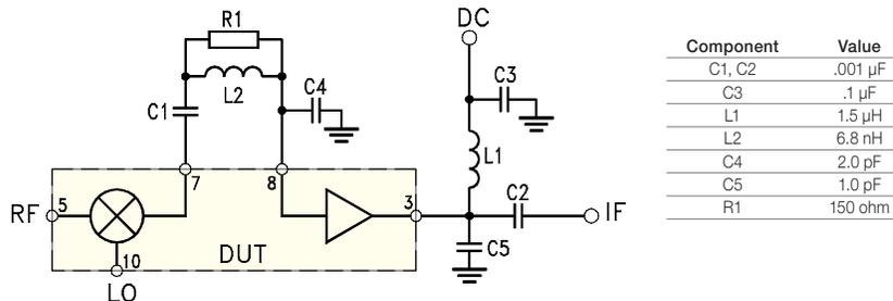
**Fig 1.** Block Diagram of Test Circuit used for characterization. (DUT soldered on Mini-Circuits Characterization Test Board TB-660+) Gain, Output power at 1dB compression (P1dB), Output IP3 (OIP3) are measured using R&S Network Analyzer ZVA-24. Noise Figure measured using Agilent's N8974A Noise Figure Analyzer
