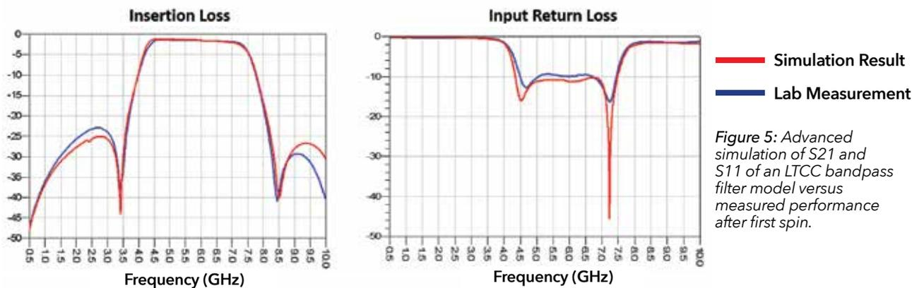
**Figure 5: Advanced simulation of S21 and S11 of an LTCC bandpass filter model versus measured performance after first spin.**
