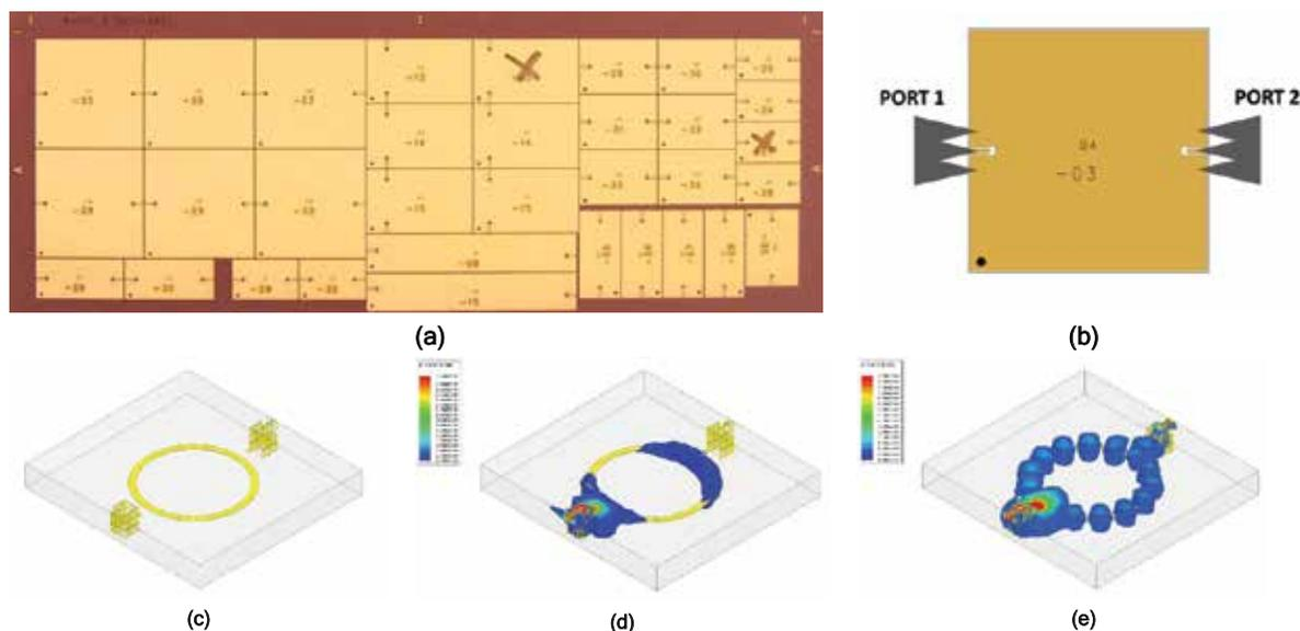
Figure 1: (a) LTCC panel with test coupons. (b) Diagram of measurement setup with RF probes. (c) 3D model of ring resonator (top and bottom layers hidden). (d) Ring resonator: E-Field plot of 1st harmonic. (e) Ring resonator: E-Field plot of 7th harmonic.
