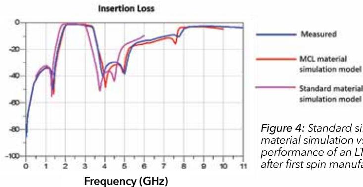
**Figure 4: Standard simulation and MCL material simulation vs. measured S21 performance of an LTCC bandpass filter after first spin manufacturing run.**
