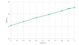
5. When ladj connection is open, Vladj =0.92V given a device with IDD=44mA Typ. For RF performance at different Vladj, please see View Data and Graph
