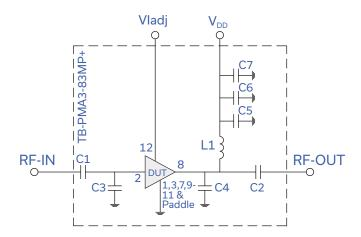
Fig 1. Application and Characterization Circuit
