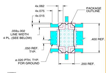
NOTES: 1. TRACE WIDTH IS SHOWN FOR ROGERS RT/DUROID5880 WITH DIELECTRIC THICKNESS 0.02"±.0015". COPPER: 1 OZ. EACH SIDE. FOR OTHER MATERIALS TRACE WIDTH MAY NEED TO BE MODIFIED. 2. BOTTOM SIDE OF THE PCB IS CONTINUOUS GROUND PLANE. DETINISTED FOR CORPER LAYOUT WITH SMOBC (SOLDER MASK
