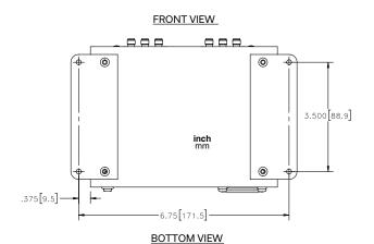
SHOWN WITH RUBBER FEET REMOVED AND BRACKETS INSTALLED.
