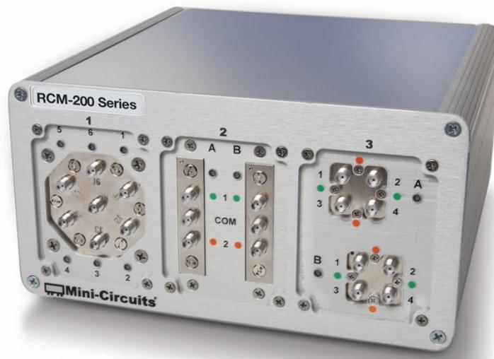
**Figure 2: Front panel of RCM-200 Series multi-function switch system, configured with 1 x SP6T, 2 x SPDT, 2 x transfer switches**
