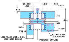
NOTES: 1. TRACE WIDTH IS SHOWN FOR ROGERS RO4350B WITH DIELECTRIC THICKNESS .030" ± .002"; COPPER: 1/2 OZ. EACH SIDE. FOR OTHER MATERIALS TRACE WIDTH MAY NEED TO BE MODIFIED. 2. BOTTOM SIDE OF THE PCB IS CONTINUOUS GROUND PLANE.
