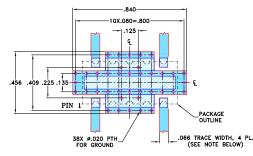
NOTE: 1. TRACE WIDTH IS SHOWN FOR ROGERS RO4350B WITH DIELECTRIC THICKNESS .030"±.002"; COPPER: 1/2 02. EACH SIDE. FOR OTHER MATERIALS TRACE WIDTH MAY NEED TO BE MODIFIED. 2. BOTTOM SIDE OF THE PCB IS CONTINUOUS GROUND PLANE.
