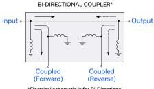
\*Electrical schematic is for Bi-Directional coupler with internal transformer(s) that routes DC from all ports to ground
