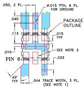
TRACE WIDTH IS SHOWN FOR ROGERS R04350B WITH DIELECTRIC THICKNESS .020" ± .0015"; COPPER: 1/2 OZ. ON EACH SIDE. FOR OTHER MATERIALS TRACE WIDTH MAY NEED TO BE MODIFIED.
