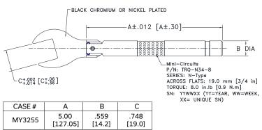
Dimensions are in inches [mm]. Tolerances: 3 Pl. ± .006 [0.150] Inch [mm]
