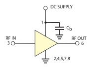
$$C_b\!\!=\!100pF$  to 10~nF Test Board includes case, connectors, and components (in bold) soldered to PCB
