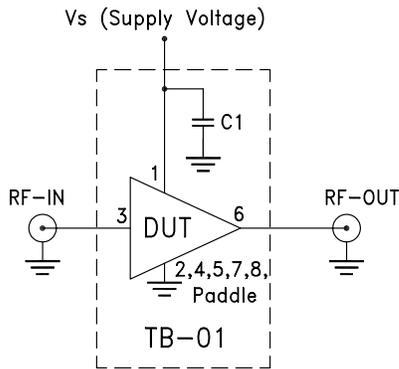
**Fig 1.** Block Diagram of Test Circuit used for characterization. (DUT soldered on Mini-Circuits Characterization test board TB-01) Gain, Return loss, Output power at 1dB compression (P1 dB), output IP3 (OIP3) and noise figure measured using Agilent's N5242A PNA-X microwave network analyzer.
