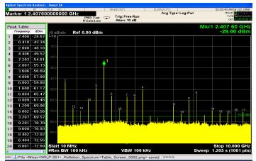
Figure 1. IF output reflection spectrum without filter
