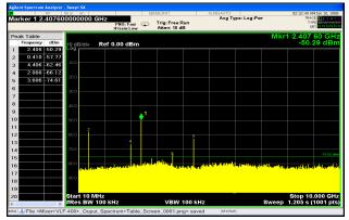
Figure 3. IF output reflection spectrum with reflectionless filter
