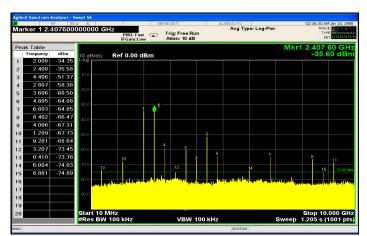
Figure 2. IF output reflection spectrum with conventional filter
