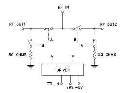
2. All RF connections must be blocked or held at 0V DC. Low frequency is determined by value of Coupling capacitors at RF ports
