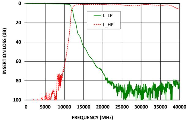
ZDSS-K10G13G+ LOW PASS PORT INSERTION LOSS (Pin=0dBm)
