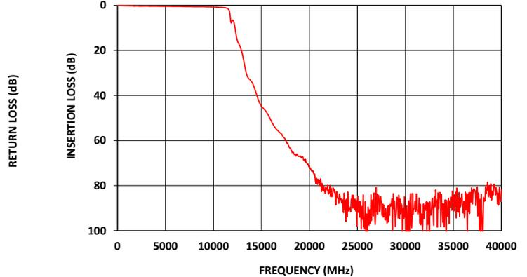
ZDSS-K10G13G+ HIGH PASS PORT INSERTION LOSS (Pin=0dBm)
