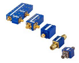
Mini-Circuits' Suspended Substrate Stripline filters offer low insertion loss by implementing printed circuit board suspended between two parallel ground planes, providing high Q. Low insertion loss combined with wide stopband makes them an excellent choice for wideband instruments and systems like ECM, ECCM, ELINT and ultrabroadband receivers.
