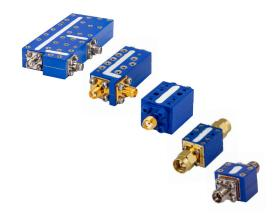
Mini-Circuits' Suspended Substrate Stripline filters offer low insertion loss by implementing printed circuit board suspended between two parallel ground planes, providing high Q. Low insertion loss combined with wide stopband makes them an excellent choice for wideband instruments and systems like ECM, ECCM, ELINT and ultrabroadband receivers.
