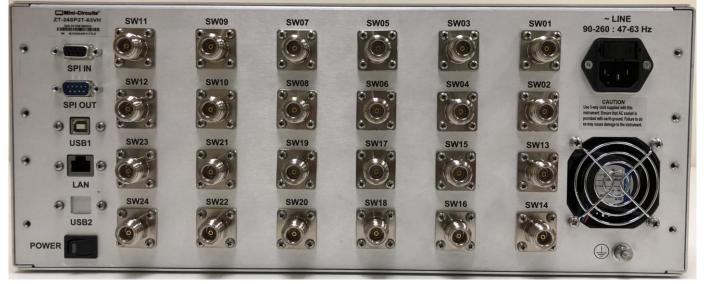
Each USB-1SP2T-63VHX module (24 total) will be controlled as a single SPDT switch with 3 states:
