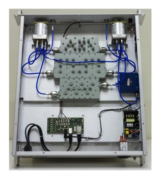
ZT-254 is a compact, rack-mounted, filter bank capable of housing up to 6 switched channels. Filter choices can be made from any of Mini-Circuits' 100s of catalog or custom models, and third-party supplied filters can also be accommodated.
