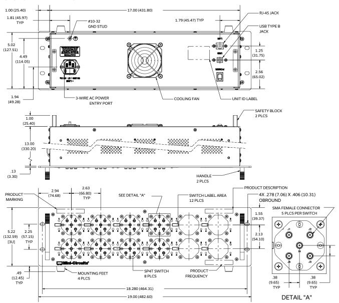
Dimensions are in inches (mm). Tolerances: ±2 Pl. inch; ±3 Pl. inch. Weight: 5700 grams.
