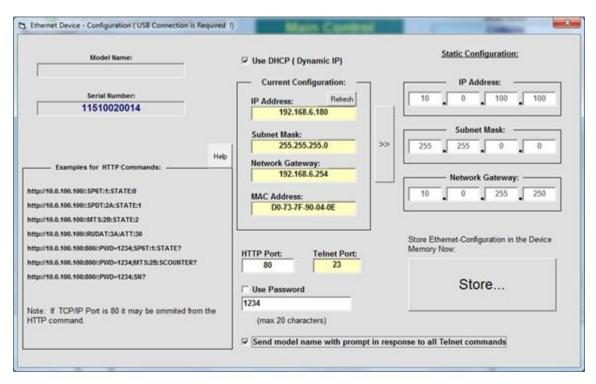
Figure 29: Ethernet configuration screen
