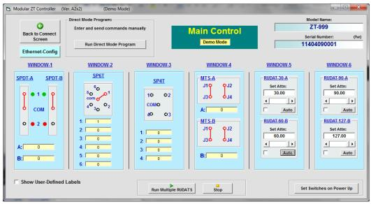
Figure 21: Example ZTM GUI main control
