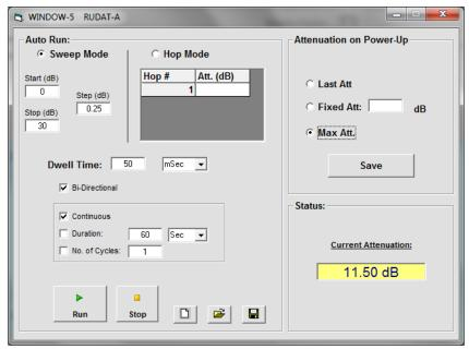
Figure 26: Attenuator sequencing menu
