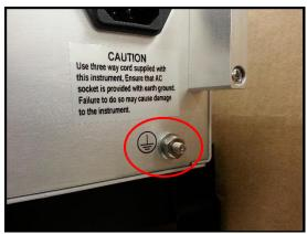
Figure 8: Rear panel grounding terminal
