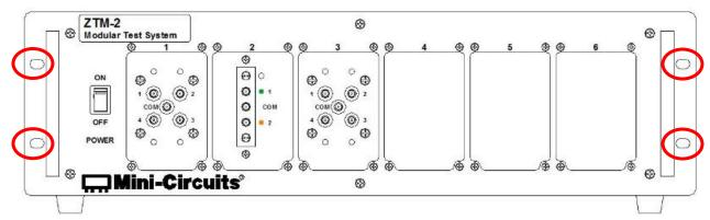
Figure 7: Slotted rack mounting holes in front panel of ZTM equipment chassis
