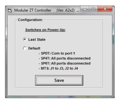
Figure 25: Power-Up Switch State menu
