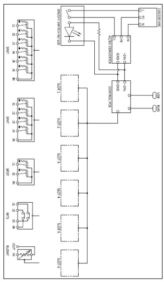
Figure 4: ZTM-series modular test system block diagram
