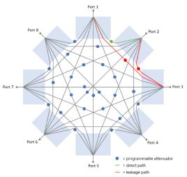
The green path in the diagram opposite is the direct path between ports 1 & 2. In an ideal mesh this would be the only route between these 2 ports. The insertion loss (IL) on the green direct path is approximately as below, when the attenuator highlighted in green is set to 0 dB:
