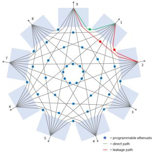
The green path in the diagram opposite is the direct path between ports 1 & 2. In an ideal mesh this would be the only route between these 2 ports. The insertion loss (IL) on the green direct path is approximately as below, when the attenuator highlighted in green is set to 0 dB:
